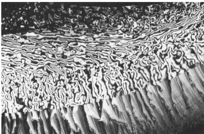
FIGURE 6 Lyotropic mesophase: columnar nematic schlieren texture N_c between isotropic liquid and discotic hexagonal phase D_h at room temperature of compound 9 in EMMac (See Color Plate IV at the back of this issue)
